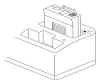
2. The batteries are charged in 14-16 hours. The charge indicator will turn into green with the charge process is completed.
